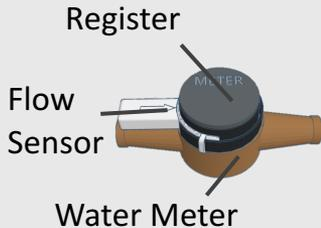
Then, secure Flow Sensor around water meter's Register. Register is typically black and fastened to the top of the metal water meter. Ensure the Water Hero Logo is facing up
